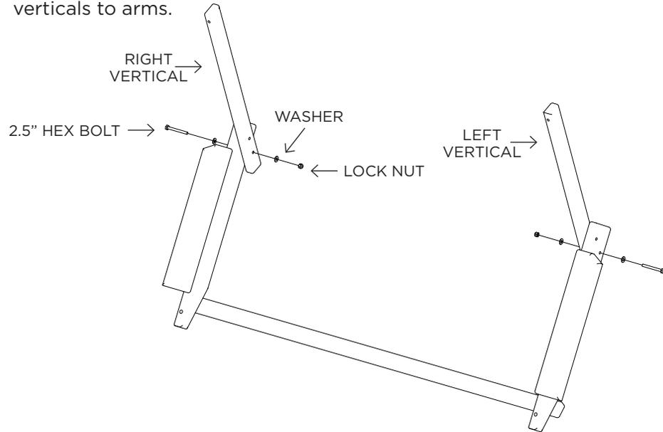
**STEP 3.** Attach bottom of left and right verticals with 2.5" eye bolts. (Medium Chain)
