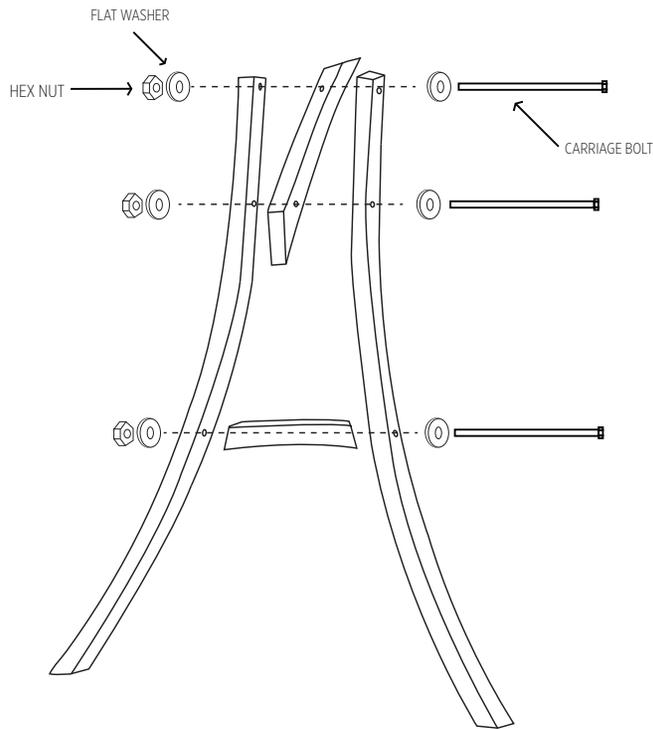
**STEP 1.** Insert (3) Hex bolts, (6) flat washers (one on each side), and (3) hex nuts into the top, middle, center section of beams. Repeat on each side. The top center beam should hand lose until step 2.
