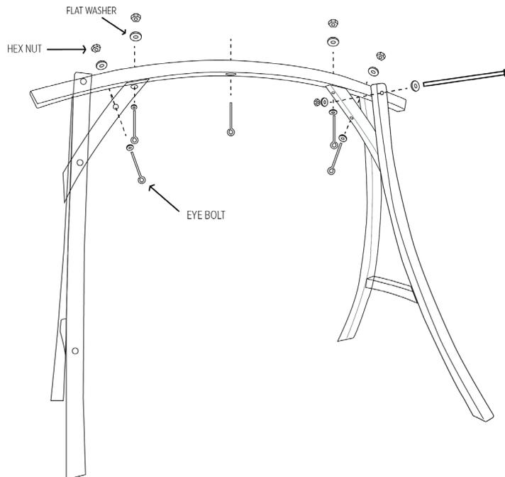
**NOTE.** Recommended use of the (8) rubber/plastic caps provided, to cover the exposed ends of the eye bolt and hex bolts
