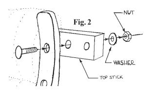
a 2 1/2" carriage bolt through the arm's top hole then through the second hole from the end of the top stick. (See Fig. 2) HAND TIGHTEN ONLY using a washer and a nut.
