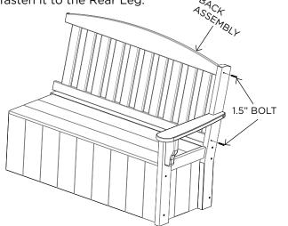
**STEP 5.** Use the Right Leg Assembly to cap off the other end. Make sure all parts are slotted correctly then use (2) 1.5" Barrel Bolts for the Back Assembly and (5) 3" Screws for the seat and panels.
