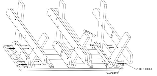
**STEP 3.** Using (1) Angled Brace at a time, slip the brace into the locating pockets as shown keeping the pilot holes on the brace to the Center Leg Assembly. Use (2) 1-5/8" Screws in the pilot holes to fasten the brace to the Center Leg Assembly, then use (2) 3" Screws to fasten the brace to the Outer Leg Assembly. Repeat for the second brace.
