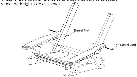
**STEP 4.** Using (2) 4.5" Barrel Bolts thread each through the bottom hole of the roll-up into the bottom hole of the upright as shown and secure using Barrel Nuts.
