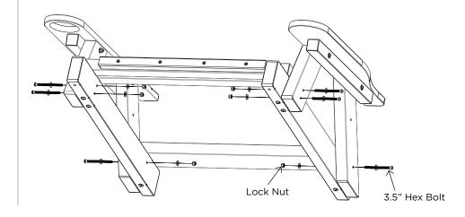
**STEP 2.** Position an upright as shown and secure it with a 3.5" Hex Bolt, a washer on each side of the material and a locknut.
