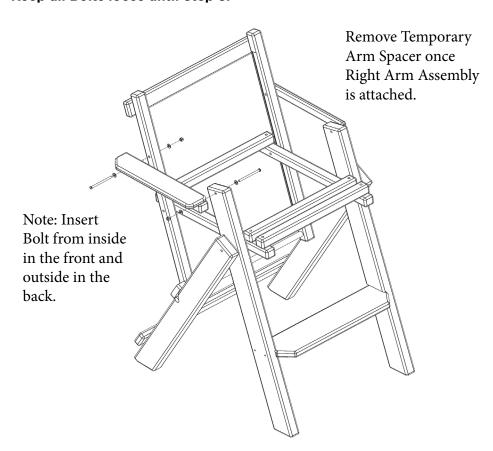
**STEP 3.** Use (2) 3.5" Hex Bolts, (2) Lock-nuts, and (4) Washers to attach Left Arm Assembly to Bar Stool Frame. **Tighten all bolts (to include existing bolts).**
