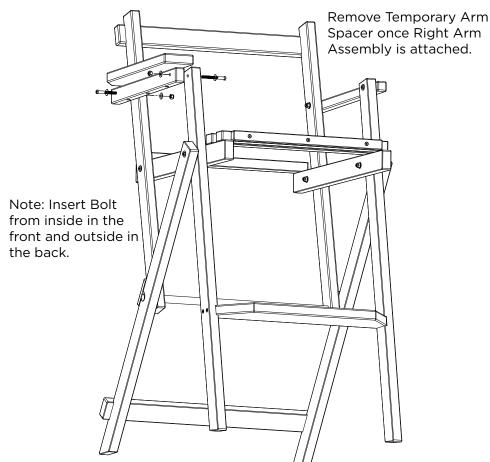
**STEP 3.** Use (2) 2.5" Hex Bolts, (2) Lock-nuts, and (4) Washers to attach Left Arm Assembly to Bar Stool Frame.
