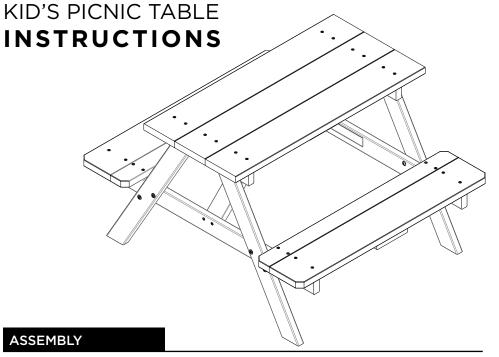
**STEP 1.** Flip Table Top over. Align the legs with the support braces on the table top. Using (4) 1.75" Hex Bolts insert the bolt through a washer, through the material as shown then secure using (1) Barrel Nut. **Tighten all bolts.**
