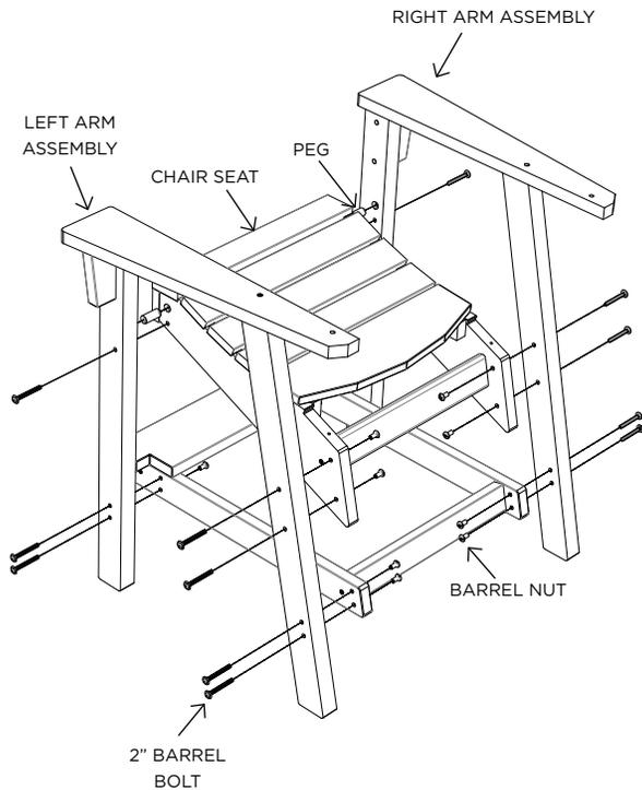
**STEP 2.** Use (2) 1.5" barrel bolts and barrel nuts to attach chair back to right and left arm assemblies.
