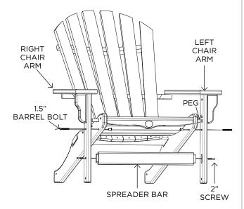
**STEP 3.** Use (2) 1.5" barrel bolts and (2) barrel nuts to attach right & left chair arm to chair back.
