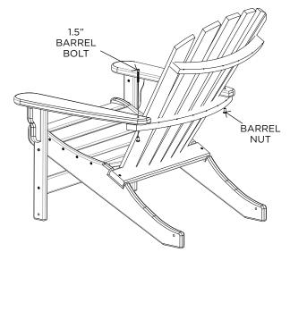
**STEP 4.** Use (4) 1.5" barrel bolts and (4) barrel nuts to attach left and right runners to chair seat and chair arms. Tighten all bolts.
