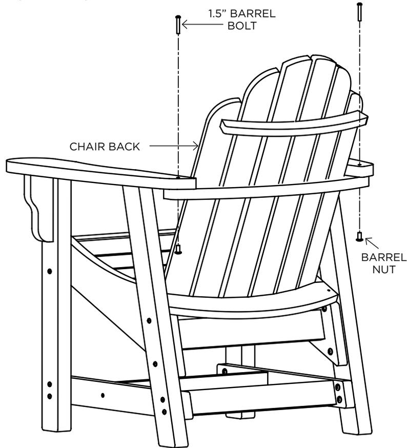
**STEP 3. PUSH FORWARD TO NOTCH IN FRAME.** Use (2) 2" torx screws to attach chair back to chair seat. Tighten all bolts once screws are in.
