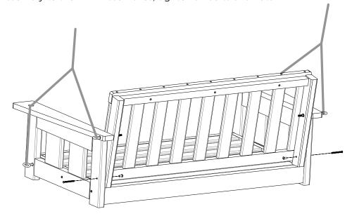
**Note:** Chain displayed upright for visibility, do not hang chain from ceiling mount until installation is complete.
