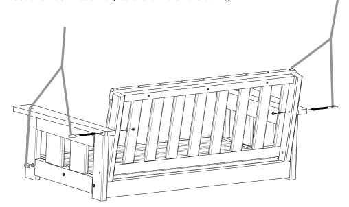
**STEP 2b.** Use (2) 2.5" Barrel Bolts to connect the bottom of the Back Assembly to the Arm Assemblies, tighten all bolts and nuts.
