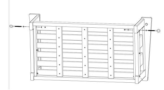
**STEP 2a.** Position the Back Assembly, use remaining eye bolts to connect the Back Assembly to the arms of the swing.
