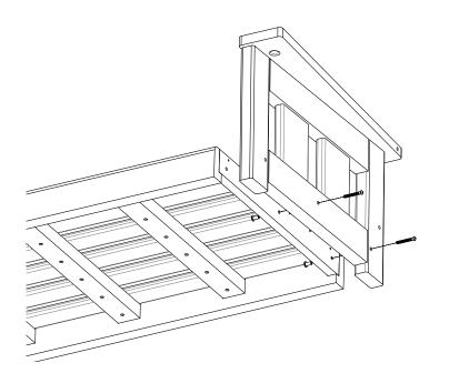
STEP 1b. After both Arm Assemblies are attached use the eyebolts connected to a chain running through the arm to tighten the arm assemblies to the seat base. Tighten the hardware.
