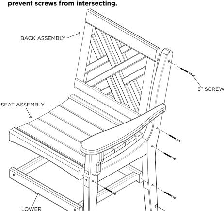
**STEP 2.** Use (6) 3" screws to attach the Right Leg Assembly to the Seat Assembly, Lower Frame, and Back Assembly.
