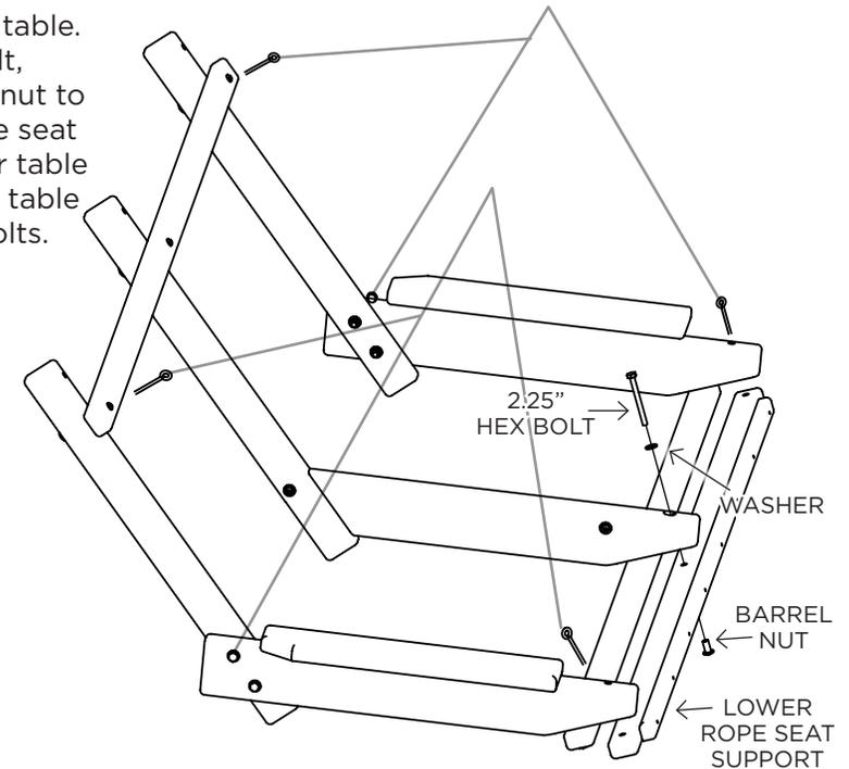
**STEP 5.** Use 2.5" barrel bolt and bolt nut to attach upper rope seat outside and middle verticals. Use (2) eye bolts, (4) washers, and (2) nuts to attach shorter end of chain set to upper seat support. Use (2) eye bolts, (4) washers, and (2) nuts to attach longer end of chain set to left and right arms. **(Rope not pictured)**
