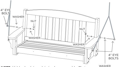
**NOTE.** Hidden back two slats to show assembly. Chain displayed upright for visibility, do not hang chain from ceiling mount until instillation is complete.
