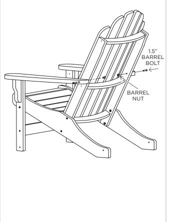
**STEP 4.** Use (4) 1.5" barrel bolts and (4) barrel nuts to attach left and right runners to chair seat and chair arms. Tighten all bolts.
