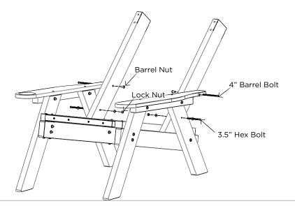
**STEP 3.** Insert (4) 4.5" Barrel Bolts, 2 per side in top hole of roll-up. Align with top holes in upright. Secure roll-up using Barrel Bolts and Barrel Nuts. Tighten all bolts, insert cup holder and enjoy!
