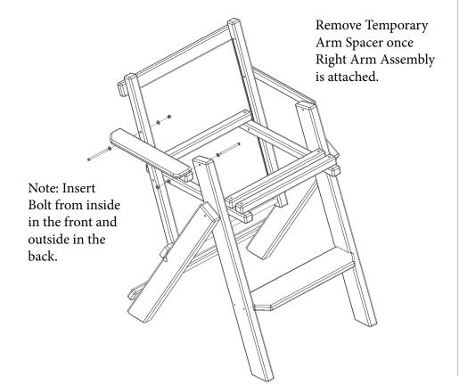
**STEP 3.** Use (2) 2.5" Hex Bolts, (2) Lock-nuts, and (4) Washers to attach Left Arm Assembly to Bar Stool Frame.
