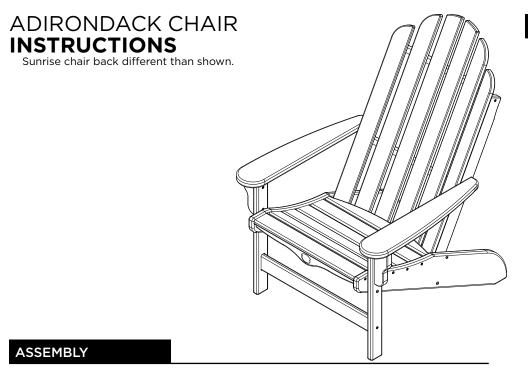
**STEP 1.** Use (4) 1.5" barrel bolts to attach chair back to chair seat. **Keep all barrel bolts loose until Step 3.**
