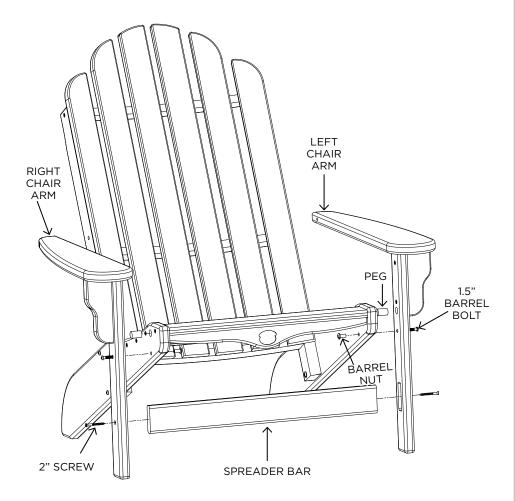
**STEP 3.** Use (2) 1.5" barrel bolts and (2) barrel nuts to attach right & left chair arm to chair back. Tighten all bolts.
